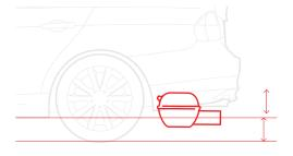
Do not install speaker acoustic system lower than vehicle's road clearance
