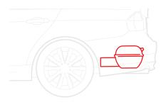
Do not install speaker acoustic system in the direction of vehicle motion
